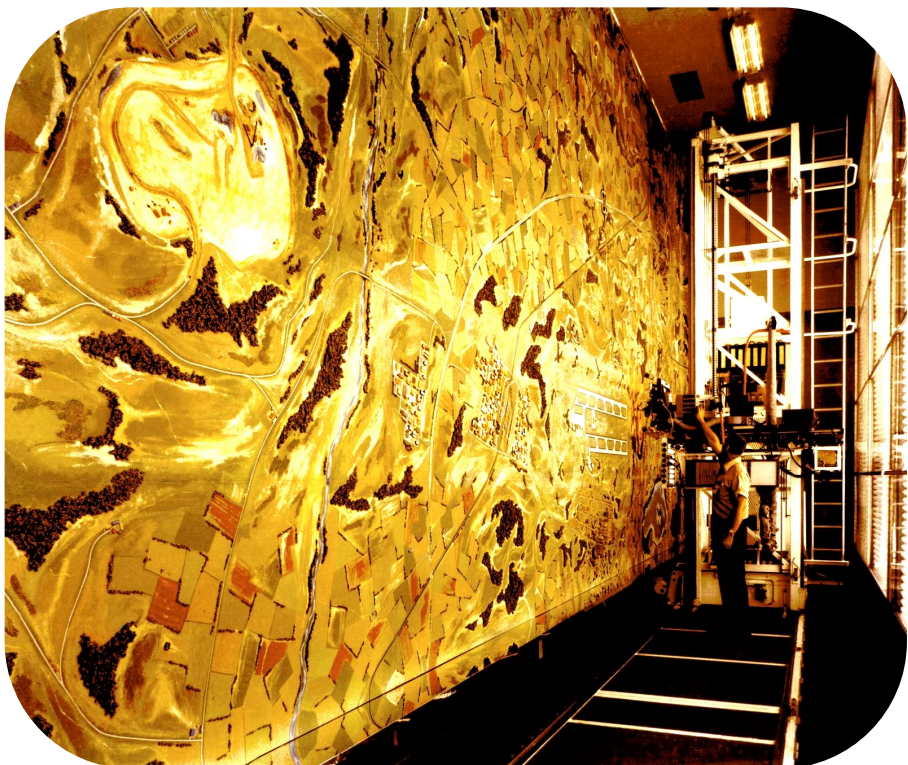
DC-8 wall terrain layout with a moving camera which appears to be just over the parallel runways on the board. Courtesy of UAHF .
