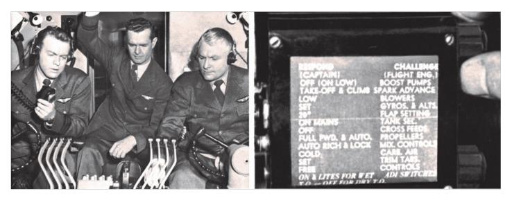
A "Challenge and Response" check was the last inspection of the DC-6's instruments and controls after the engines were run-up to cruise power prior to take-off. The scroll shows a portion of the "oral challenges" made by the Flight Engineer and "responded to" by the Captain as he made the required checks. After
