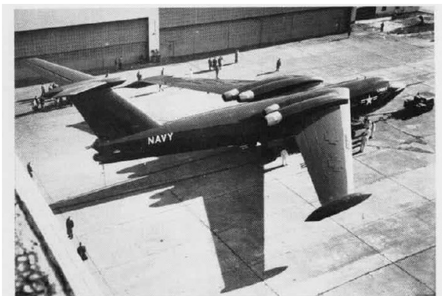
THE NAVY and Martin Aircraft unveiled the radically new XP6M-1 seaplane in January. The big aircraft is powered by four Allison J-71 turbojet engines with take-off afterburners and is capable of speeds over 600-mph. The Seamaster will cruise at 40,000 feet and will carry a 15-ton payload. New hull, T-tail, and inverted dihedral in wings, are features.
